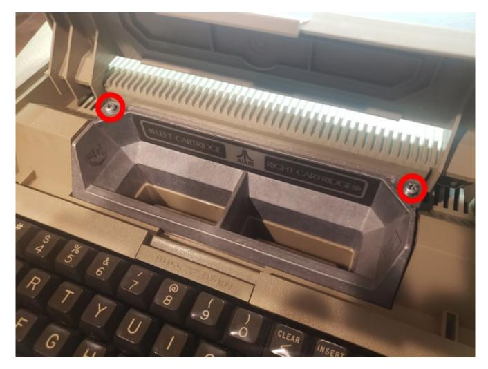
With the screws removed you can pull the top of the case forward slightly and then lift up. Set this aside.
