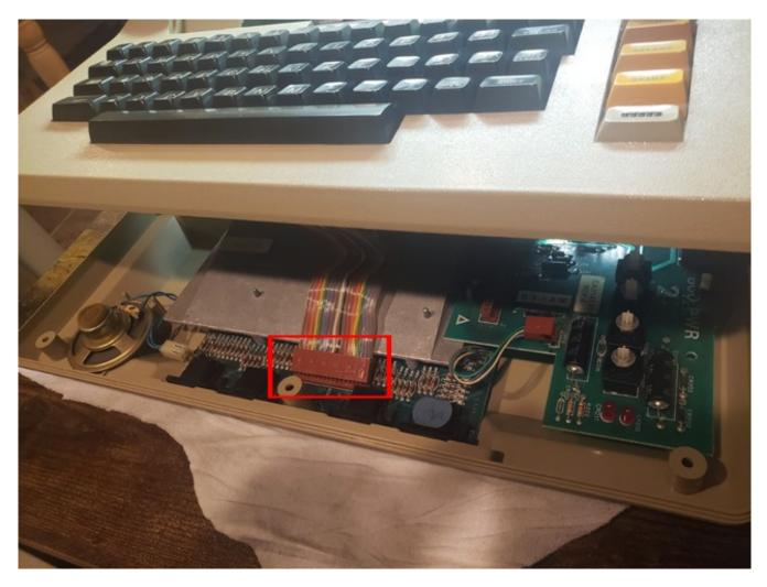
Set the bottom half of the computer aside as we'll be working only with the top half for now. Turn the keyboard/top-half of Atari upside down and remove the screws which are securing your old keyboard to the case. There may be washers under some of the screws.
