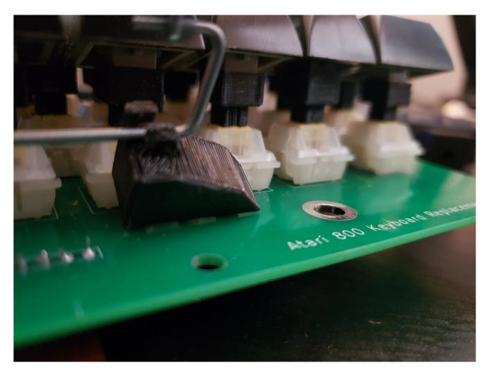
Then rotate the boot to line up with the holes on the PCB and push the pegs on the bottom of the boot through the holes on the PCB and attach the boot-lock on the underside of the PCB.
