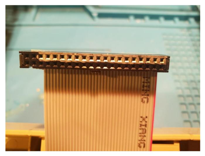
Be sure there is no twist in the cable and align the connector on the end of the ribbon cable with the keyboard connector pins.
